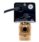
Power supply/ Frequency: 230 V AC/ 50 - 60 Hz Power consumption: 7 VA Kvs coefficient: 6.5 m³/h Operating condition of actuator: 0 - 60°C Running time (motor): 18 s Running time (return spring): 5 s Degree of protection: IP 20
